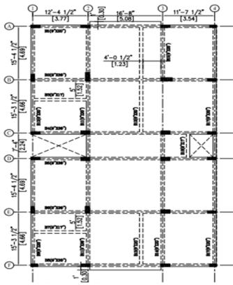
Fig1. Stilt Floor Framing Plan.
