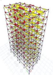
Fig4. Shear force for whole structure
