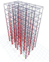
Fig5. Axial force for whole structure
