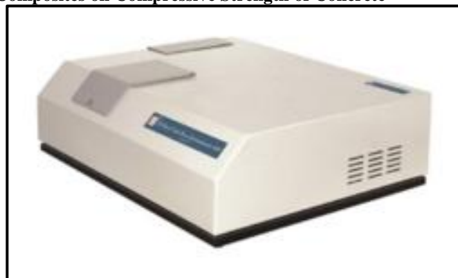
Fig 17: Systronics Double Beam UV Spectrophotometer - 2201
