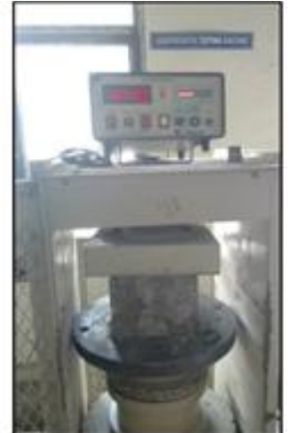
Fig 44: Compression Testing Machine (CTM) Testing the cube in CTM.
