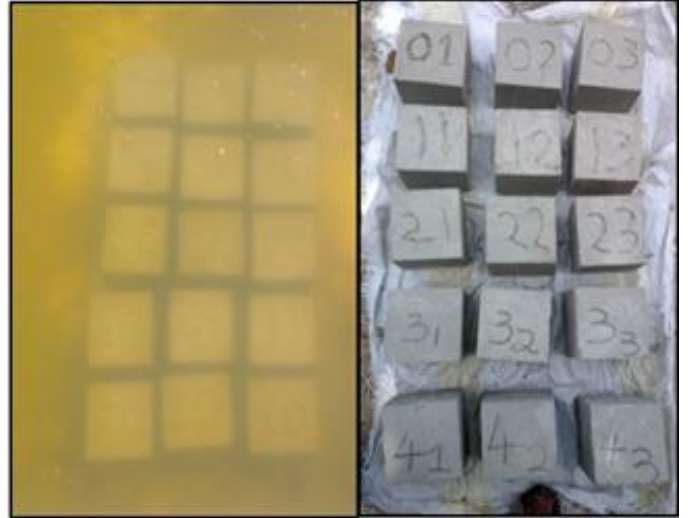
Fig 42: Curing the cubes in water After curing.
