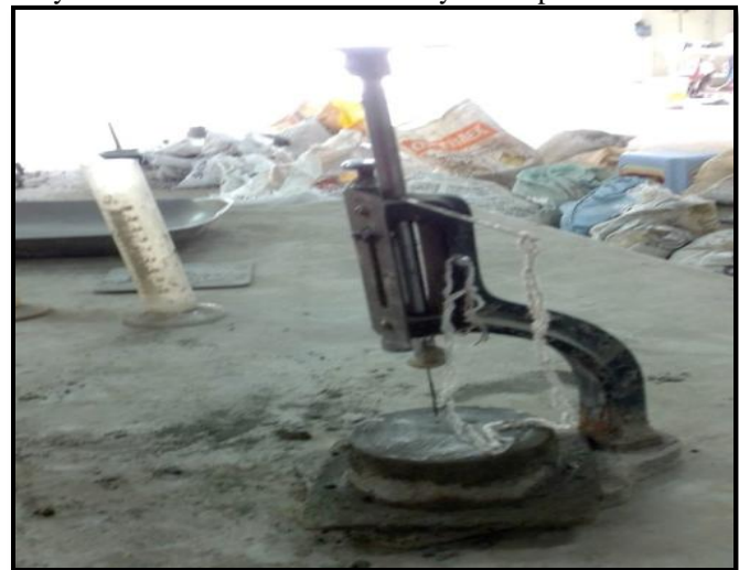
Fig 21: Vicat mould setup for 53-grade cement
