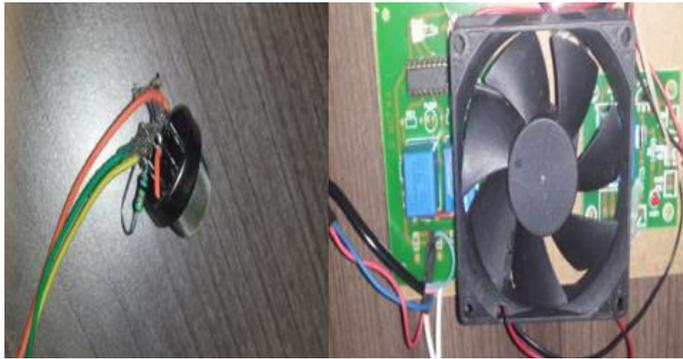
Fig.2.MQ2 Gas sensor and Exhaust Fan.
