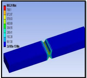
Fig.23. Heat Flux on the welded pieces.
