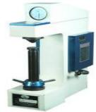
Fig.11. Brinell/Rockwell hardness tester. International Journal of Innovative Technologies Volume.06, Issue No.01, January-June, 2018, Pages: 0429-0437
