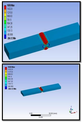
Fig.19.Temperature distribution on the welded pieces.
