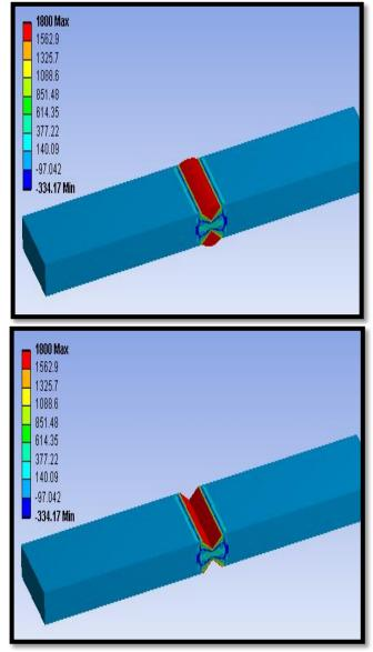
Fig.22. Temperature distribution on the welded pieces.
