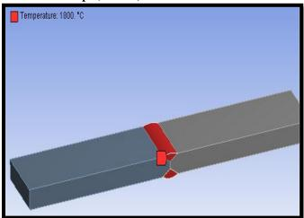
on on the welded pieces. Fig.21. Temperature is applied at the welded region. International Journal of Innovative Technologies Volume.06, Issue No.01, January-June, 2018, Pages: 0429-0437
