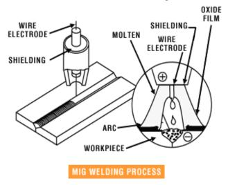
Fig.1 MIG welding process.
