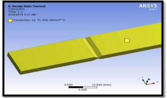
Fig.14. Applying of convection.
