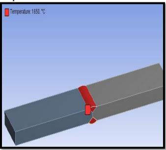
Fig.18.Applied Temperature at the welded region.
