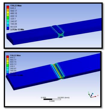
Fig.17. Heat Flux on the welded pieces.
